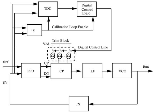
Fig. 3: Block diagram of the proposed calibration system
