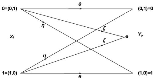
Figure 5: GEC wireless channel model graphical representation.
